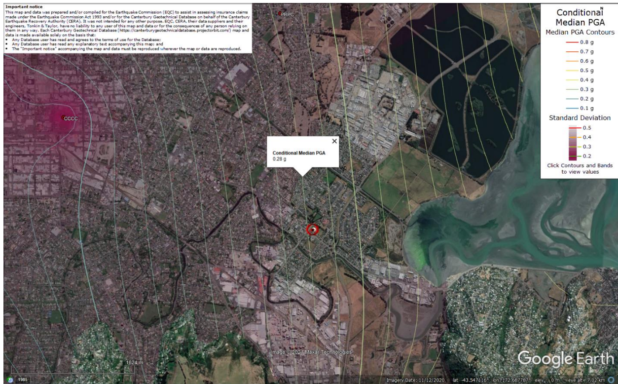
Figure 38: PGA for Dec-11 EQ (st. dev. = 0.425-0.450 ln units).
