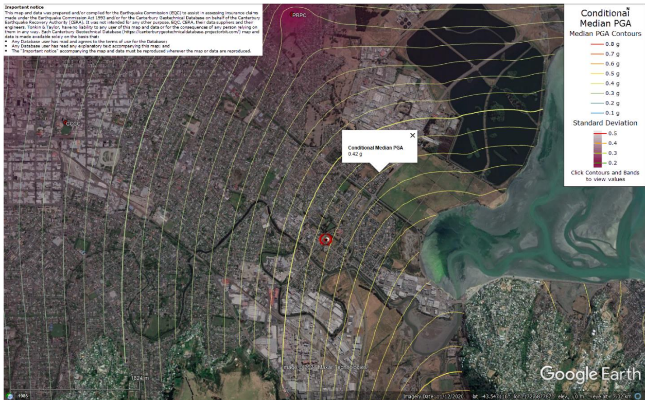
Figure 37: PGA for Jun-11 EQ (st. dev. = 0.400-0.425 ln units).
